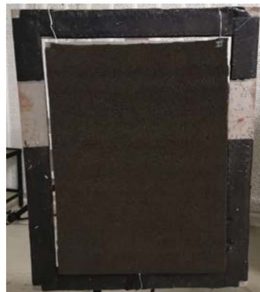
Figure 4. Photography of the foam suspended very close to the vertical plate.
